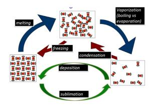
others, creating a vapor. When the pressure of the vapor = pressure above, the liquid boils.
